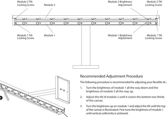
Adjust the overall brightness using the dimmer switch. 4.
